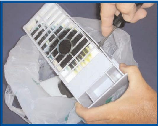
When the control panel on your printer instructs you to change the tank, remove full tank and replace it with a spare tank. Be sure to save your original box and plastic bag. With a knife, letter opener, or small screwdriver, POP off the TOP plastic cage on the tank by prying gently. It snaps out very easy! Set aside & save this.
